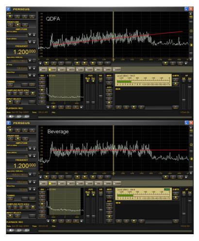
Compared to a beverage, which has uniform sensitivity over the frequency spectrum, the QDFA sensitivity tends to roll off as frequency decreases. Placing additional preamps in the phaser will increase low frequency sensitivity.
