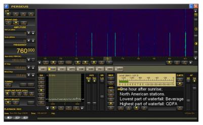
This screendump with the Perseus centered on 790 and a 100 kHz frequency span, illustrates the point above, and also illustrates that after sunrise, the beverage is far more sensitive than the Kongsfjord QDFA. The lower part of the waterfall shows mostly audible North American stations (810 is Scotland) while on the QDFA you can only see traces of their carriers.
