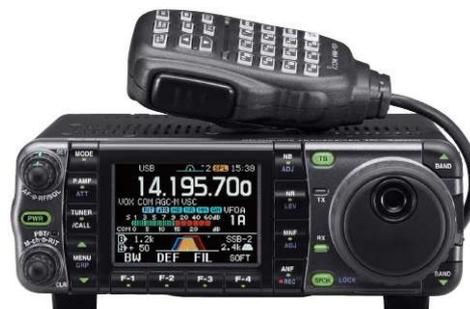
It is very small. Well, since I already have an IC-703 I shouldn't be surprised, but fact is: It's even smaller than the IC-703. WHD is 167x58x180mm and the weight is 2.3 kg. I am a metric man so if you want lbs and inches, you do the math. Of course, power is extra. For transmit it will need 22A at 100 watts; for receive it requires 1.6A at full volume.
