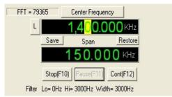
The upper display is the main tuning display, which can be set to Center Frequency (the frequency you tune to is always at the center of the Span), or Demod Frequency (any frequency within the Span you have tuned to.) Normally when you tune around, you would choose the Center Frequency.
