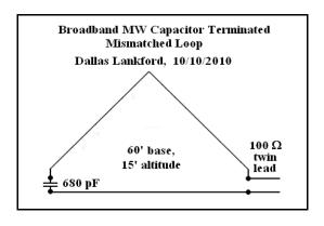
at 1490 kHz compared to a 1000 ohm terminated flag. The measurement frequencies were determined by the availability of signal sources in the direction of the antennas maximum responses. It was found that the capacitor value for a maximum in the 600 to 700 kHz range was about 680 pF.
