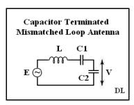
above, resonance is f = 889 kHz. This is much too high based on measurements above of signal levels for the actual antennas. So it seems that a more elaborate model is needed for better theoretical agreement with measurements.
