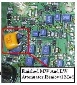
because only my finger was holding it in place). The finished mod is shown in the photo above. The photo is about 2.5X magnification (when the article is printed on an 8.5 by 11 page), which gives you an idea of how tiny the parts are.
